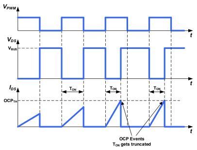
Fig. 28. OCP threshold timing diagram
