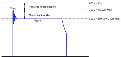
Fig. 30. QR flyback drain-to-source voltage stress diagram
