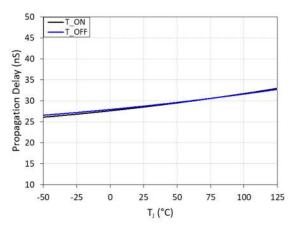
Fig. 14. Propagation delay (T<sub>ON</sub> and T<sub>OFF</sub>) vs. junction temperature(TJ)
