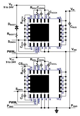
Fig. 21 Half-Bridge Configuration
