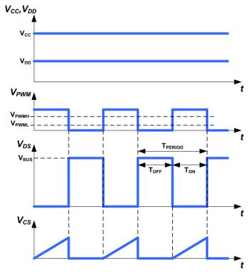
Fig. 23. Normal operating mode timing diagram
