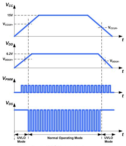
Fig. 22. UVLO Mode timing diagram
