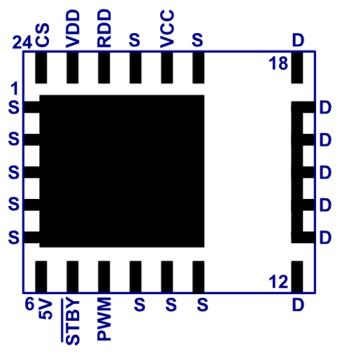
Fig. 19. Package Top View
