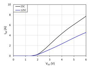
Fig. 4. Source-to-drain reverse conduction voltage
