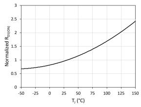
Fig. 7. Normalized on-resistance  $(R_{DS(ON)})$  vs. junction temperature  $(T_i)$
