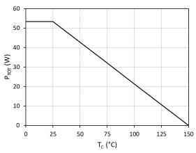
Fig. 16. Power dissipation (P<sub>TOT</sub>) vs. case temperature (T<sub>C</sub>)
