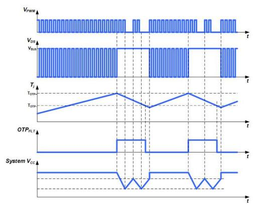
Fig. 29. OTP threshold timing diagram
